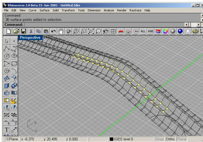
**Move** the points up 1.5 mm to smooth out the center section of the surface, and turn off the control points.
