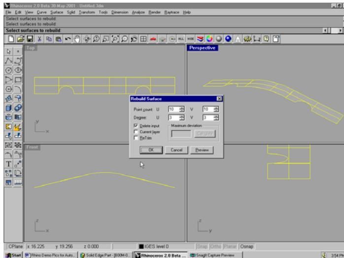
After **merging** the three surfaces into a single surface and detaching the trim curve, the new single surface is **rebuilt** to increase the number of control points for editing. In this case the middle four rows of control points are moved up 1.5mm to create a raised center section.
