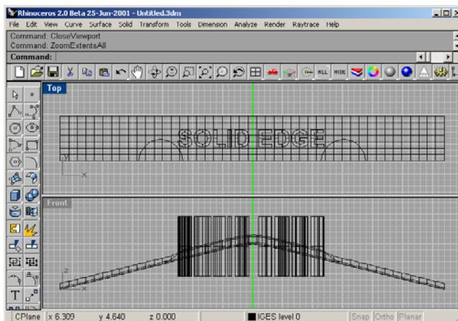
Use the **BooleanDifference** command to subtract the lower part of the text characters from the surface.
