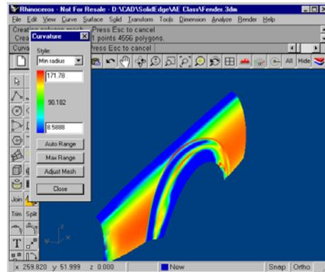
*Curvature analysis shows the curvature values of the surface in color.*
