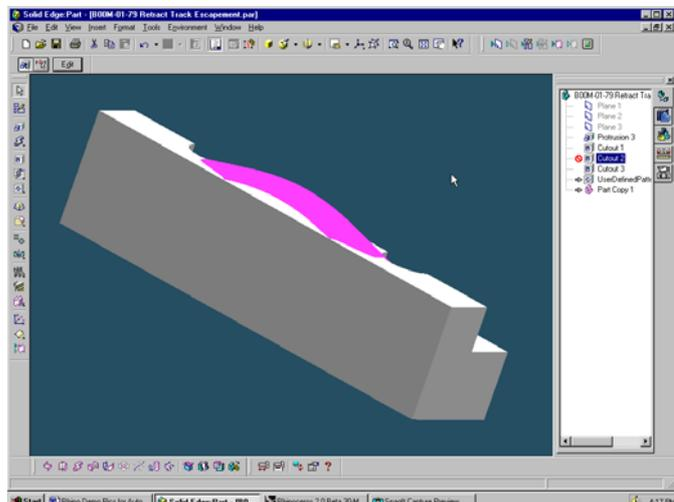
The part copy is then used to **replace** the face of the solid body.
